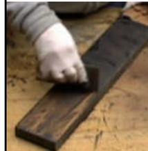
Use a cabinet scraper to remove excess. Don't let filler dry too long before removing.
