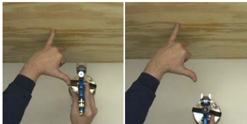
Too Close - Running & Sagging
