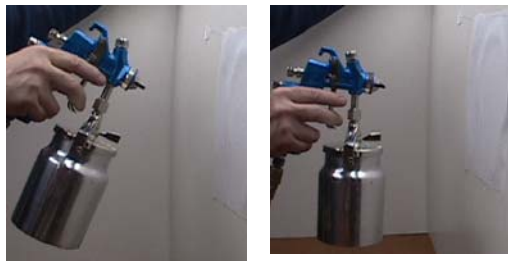
Tipping the gun results in more finish at the bottom of the pattern than at the top
